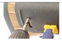
4. Using a  $\frac{1}{4}$ " drill bit, carefully enlarge the holes that were previously drilled with the 3/16" drill bit.
