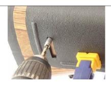
3. Place drill bushing against upper inside edge of slot as shown. Carefully drill HALF WAY through stock. Repeat with remaining 3 slots.
