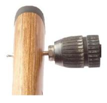
5. After enlarging the holes with ¼" drill bit, remove the cheek riser from the stock and connect each pair of holes by drilling completely through the stock from one side to the other.
